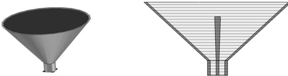
**Figure 4:** Optimized antenna (left), vertical cut of the optimized antenna (right).
