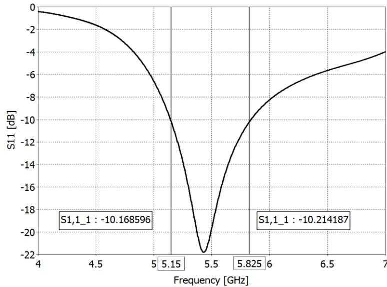
**Figure 5:** Frequency response of return loss of the optimized antenna.
