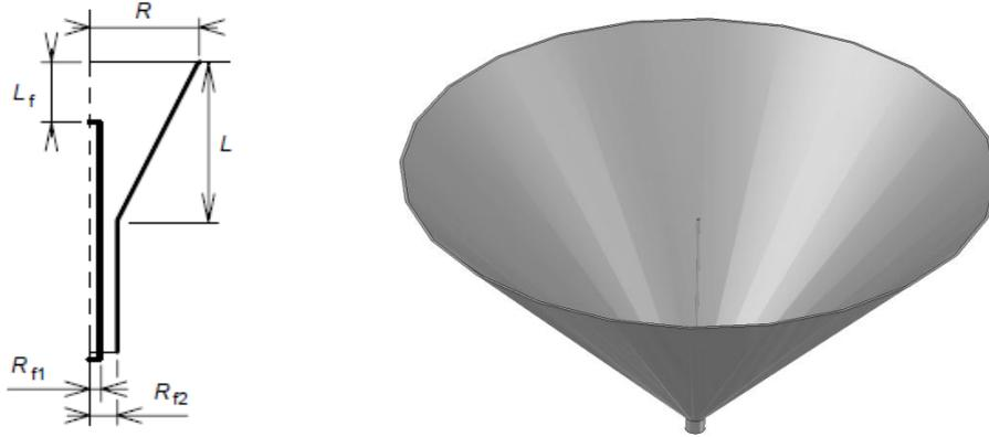
**Figure 1:** Vertical cut of the antenna (left), modeled antenna (right).
