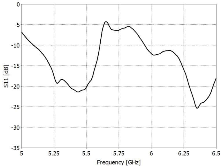
**Figure 2:** Frequency response of the return loss of the antenna.
