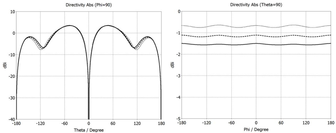
**Figure 6:** Radiation pattern of the antenna in E plane (left), H plane (right), (5.2GHz – solid, 5.43GHz – dashed, 5.8GHz - dotted).
